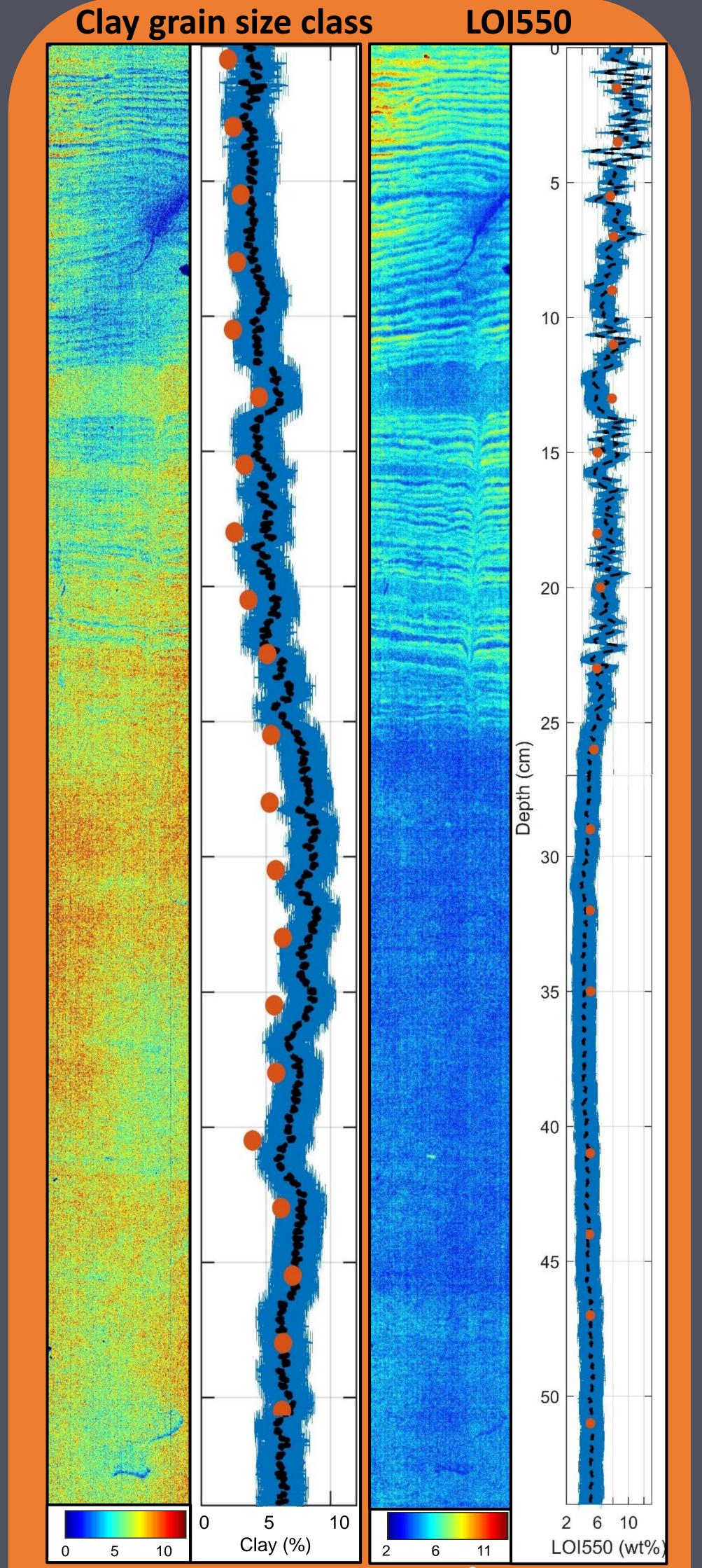
Determination coefficient R<sup>2</sup> of the two SWIR models are 0.79 (Clay grain size class, n=21, 5LVs) and 0.76 (LOI550, n=19, 5 LVs). Average predictions (dark) are compared to the reference values (orange point) and seems to follow the same trend. Variations inside each stratigraphic unit event at the scale of laminae can be studied at 189µm.
