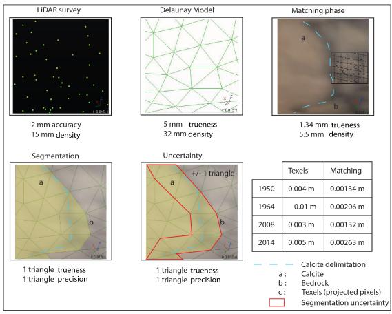
Fig. 5. LIDAR survey, meshing process and the calculation of the uncertainties. Considering: i) the uncertainty produced by the mesh construction; ii) the photo draping and iii) the digitising process, the matching uncertainty reaches 2.6 cm for the 2014 photograph. It is smaller than the mean 0.032 m triangle size of the mesh. Consequently, because of the resolution that was used for the mesh, the cutting process generates larger uncertainties than the draping method.
